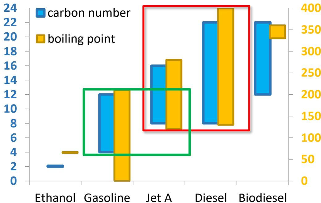
Distillation cuts based on boiling point, determines product slate
